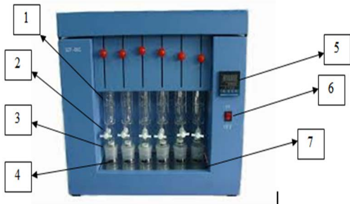
Fig. 1: Soxhlet extraction apparatus, (1) Condenser pipe, (2) Cock, (3) Extractor, (4) Extraction flask, (5) Temperature Indicator, (6) Power switch, (7) Water bath.
